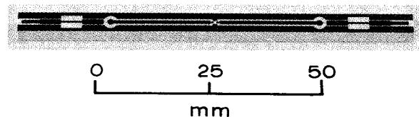
Figure 4. Coplanar waveguide circuit.
