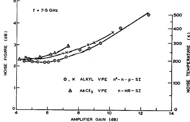
Figure 5. Single stage amplifier results for three devices, each from a different slice.
