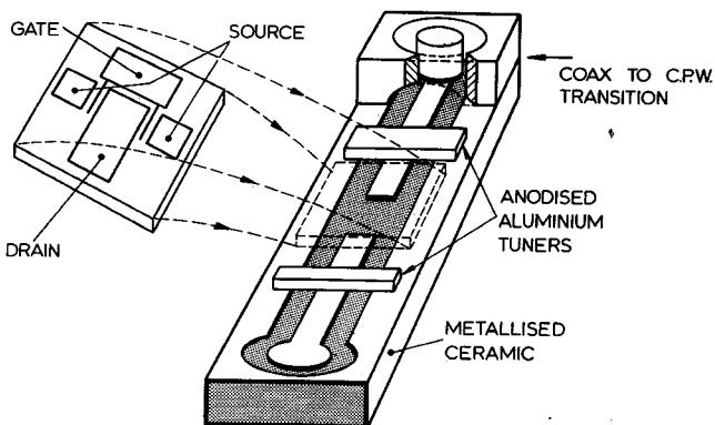
Figure 3. Schematic view of chip and coplanar waveguide circuit.
