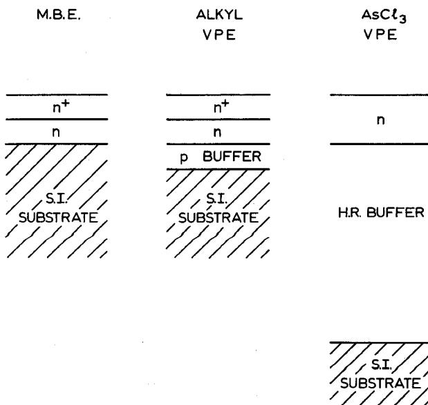
Figure 1. GaAs epitaxial growth structures.
