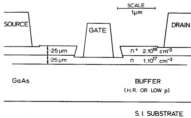
Figure 2. Cross section of active region of typical FET.
